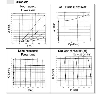
The fluid used is a mineral based oil with a viscosity of  $46 \text{ mm}^2/\text{s}$  at  $40^\circ\text{C}$ . The tests have been carried out at with a fluid of a  $40^\circ\text{C}$ .
