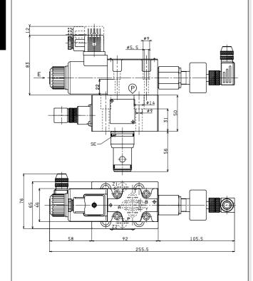
Fixing screws T.C.E.I. M8X45 UNI 5931
