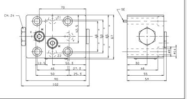
Weight: 2,1 Kg **M** = pressure gauge attachment
